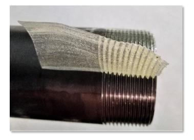
Remove masking tape while the RPC 7555 is wet. If curing has commenced, wait until the RPC 7555 is fully cured and carefully pull the masking tape 180° backward NOT at a 90° angle to the substrate surface – pulling the tape at a 90° angle may pull the tape edge of the RPC 7555 off the substrate. Lightly score the tape line with a sharp razor blade prior to pulling the masking tape off fully cured RPC 7555.
